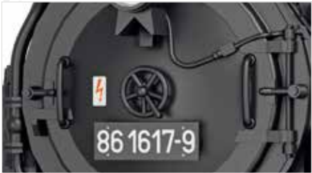
Elaborate smoke chamber door
