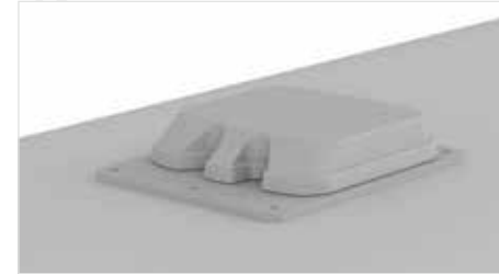
Prototypical aerial equipment on the coach roofs
