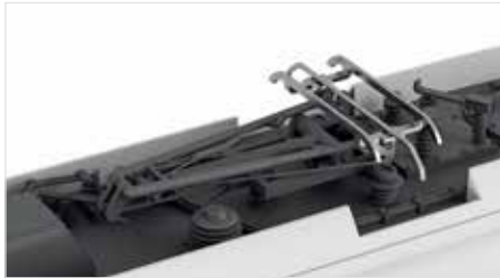
Pantograph arrangement of the class 408
