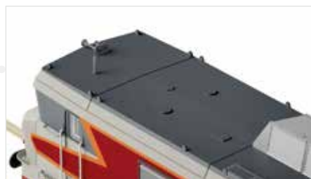
Correct realisation of the roof side without pantograph
