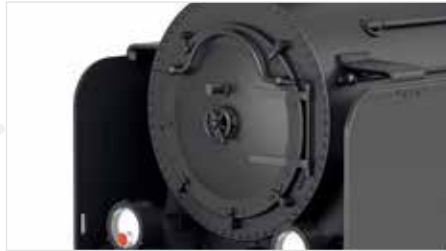
Smoke chamber with separately attached plug-in parts
