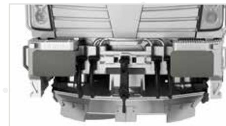
High-speed rail scraper
