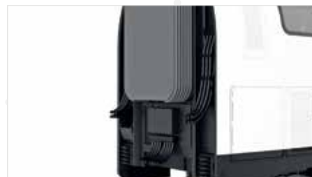
Reproduction of the cables between the coaches
