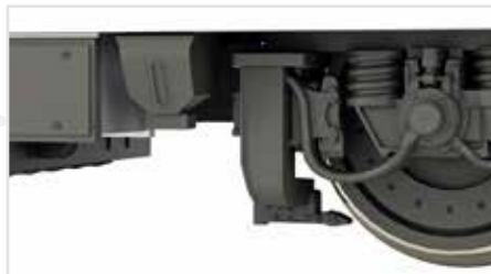
Reinforced design of the sand downpipes
