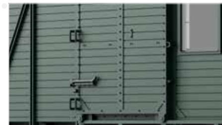
Separately attached handles and latches on the door
