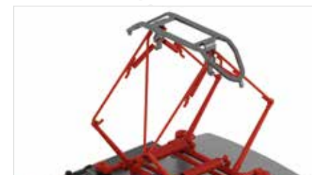
Dainty pantograph of the type RBS 58
